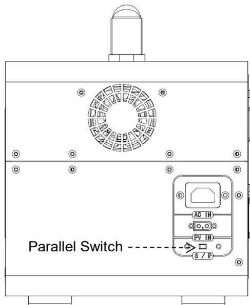
The 2<sup>nd</sup> VOLANS's output power will be 2 times rated output power of VOLANS after connected in parallel.(MAX output power can up to 2400W)
